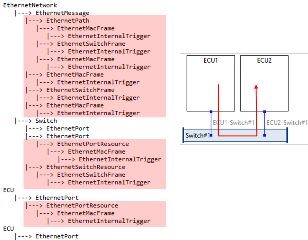
Figure 4.13: Example of a timing analysis model for a simple network with a single message.
