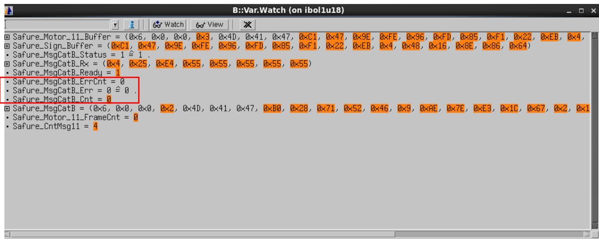
Figure 3: Correct sequence counter case (Emulator view)
